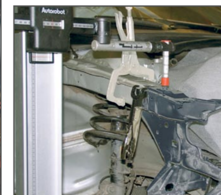
An Calipre specialty. Datasheets have measuring points for fender mounting screws, as well. These points facilitate new-part positioning before welding.
