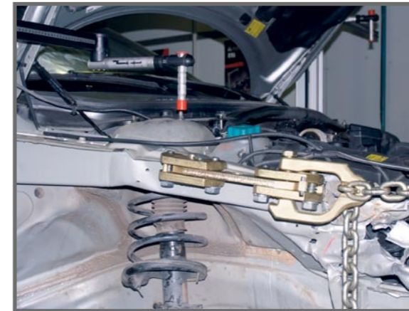
Double gripper is great for pulling reinforced metals. Place the measuring head according to the datasheet, then track how closely the repair is moving toward the target.
