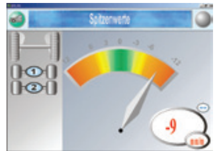
The result of the sideslip test in mm / m with coloured measured values
