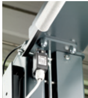
Automatic limit switch (roof protection)
