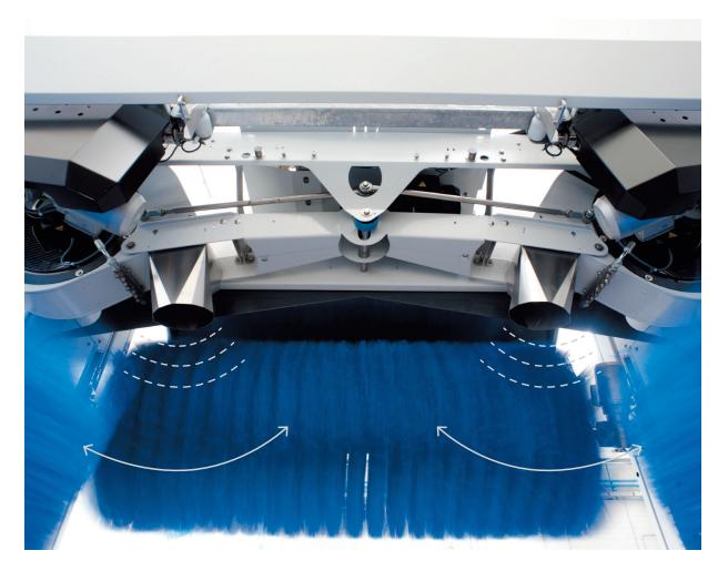
The top dryers generate **oscillating air flows with an elliptical trejectory** optimal for the natural flow of the water on the car and so down on the ground: this guarantees a great combination between wash and dry.
