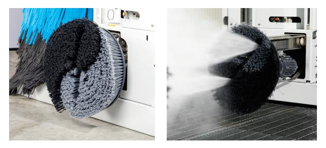
**The Wheel Master** is developed to wash the wheels, the side of the car and all lower parts of the vehicles. Operated by **two high pressure nozzles**, thanks to a great combination between power of the high pressure and the softness of the brush, Wheel Master guarantees an **excellent washing result even in difficult spots.**
