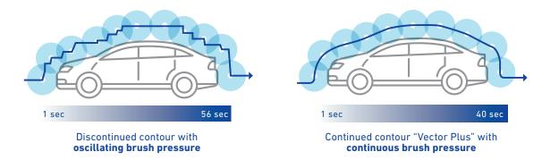
In the Hydrus Tech 2.0 a **Profile Control Tech has been implemented as a standard feature: the profile of the vehicle is contoured in detail.** The result is a more accurate washing quality with the combination of the reduced washing time mainly thanks to the introduction of INVERTERS for the control of the brushes. **The delicate touch** of the brushes is guaranteed even at high speeds.
